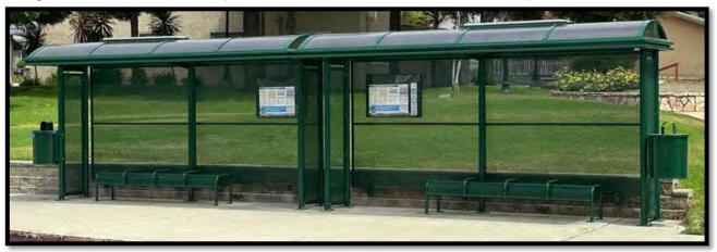
Using a consistent shelter design will help create a unified look to the system. The shelters most recently installed are13-ft. wide or 17-footwide Polycarbonate Dome Roof and perforated metal side panels with a roof mounted LED solar lighting system. The preferred panel material is vandal resistant perforated metal rather than tempered glass or Plexiglas. Perforated metal is less prone to breaking and is easier to clean. A bike rack or bike locker is considered on a case-by-case basis.
